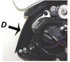
Attach the rubber lip as shown in figure D. The thin part of the lip shows to the inside.
