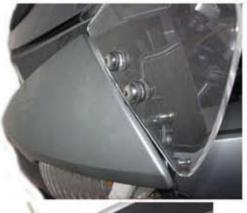
Insert the rubber grommets to the wind deflector and install the handguard to the vehicle using the delivered carriage bolts and the special nuts.
