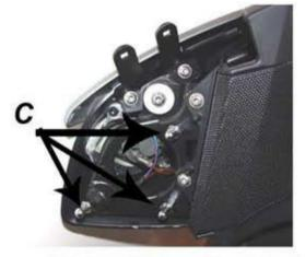
Now install the bracket (figure C) using the delivered M6 screws.
