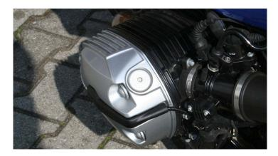
Oil filler plug Torx, made of high-quality aluminium. Use a Torx tool T45 from your BMW tools in order to fit and remove the oil filler plug. Choose between the anodized and the black anodized version (see Torx tools).
