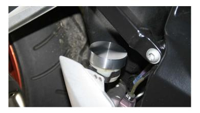
Cover for the foot brake fluid reservoir, CNC machined of aluminium. Image shows K1200R, but it is also visible on: K1200RS without Int. ABS K1200S R1200S, R, ST & GS R850, 1100, 1150GS & R850, 1100R If you do not have any silicone at home, you can also order our high-quality silicone which is pre-filled in the volume you need and easy to dose.
