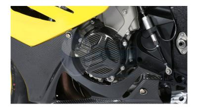
This Alternator Cover is made of high quality carbon fibre and covered with UV resistant clear lacquer. The article number LMD.029.S100S.K has an ABE/street homologation. The article number LMD.075.S1RAR.K is specially made for the race track.
