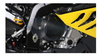
This Clutch Cover is made of high quality carbon fibre and covered with UV resistant clear lacquer. The article number KDA.031.S100S.K has an ABE/street homologation. The article number KDA.077.S1RAR.K is specially made for the race track.
