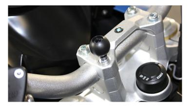
You screw the GPS ball into the upper triple clamp. The screw is 55/60/65mm long with a M8 thread. Attention: If handlebar risers are mounted, these screws are possibly too short. You can mount many different GPS mounts to it, for example RAM mounts or the mounts which we offer under Extra GPS Mount.Diameter RAM ball: 1 inch (2,54 cm)
