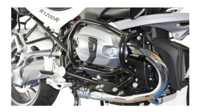
Our crash bars are made of high-quality steel and are especially designed for your R1200R 2005-2014. The crash bars are designed to be very robust and provide an equal distribution of the forces to ensure that you and your bike are protected in the best possible way. Crash bars offer a very good protection, but they can reduce the lean angle.
