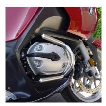
These stainless steel engine guards will never rust like powder coated steel guards. They are carefully designed to allow clearance for oil changes or valve cover access, so they never need to be removed. Guards attach to the engine mounts not the engine covers to protect the engine heads and not destroy them. Integrated top brackets on each guard allow the rider to mount accessory lights, video cameras, or whatever they can imagine! BMW R1200RT 2005-2009
