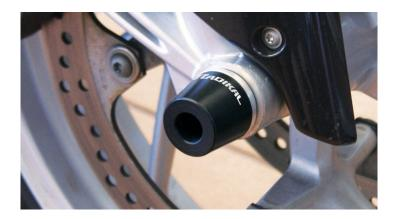
These crash protectors for forks are made of cnc lathed plastic (POM). The mounting is made of cnc milled and anodized aluminum.
