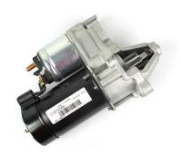
This starter made in original equipment manufacturer quality has a very high performance and a long life span. Anti CW rotation, 9 tooth, 12V 1,1 KW, magnets are glued and clamped.
