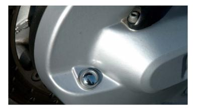
Chrome cap II was created for covering the gear oil filler screw. Like cap I it is just pushed on and fits perfectly.Not for R1200GS.
