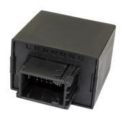
12-pin electric relay for turning signals. When using LED indicators, this relay will automatically adjust to the power of the turning signals to ensure the correct flashing rate (1-100 Watt) or for simple exchange of the original relay!
