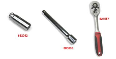
You will need a special small and long wrench socket size 14mm to remove the spark plugs of your BMW R1250 engine (article number 682062). In addition to the wrench socket you will need an extension (article number 880039) and the correct 3/8inch ratchet wrench (article number 821557).
