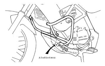
The Hepco & Becker Crashbars offer the best protection in each situation. The pipe-in-pipe construction is easy to install and the black engine guard fits prefect to your Enduro.
