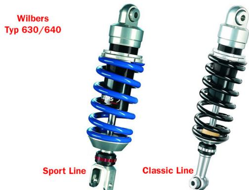
The basic Wilbers Racing Suspension shock absorber is adjustable in rebound and preload. Depending on the article number it is either the shock 630 with 36 mm diameter or the version 640 with 46 mm diameter. With many motorcycle models the shocks can be assembled individually to raise or lower the seating height. Wilbers Suspension rear without external compensating reservoir.
