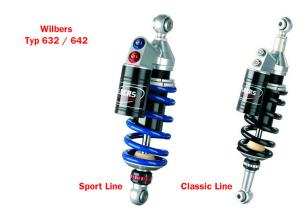
The 632 and 642 series shock is ideal for Competition use and also serves as many applications for road usage. These have lots of unique special parts including a 46mm radial flow piston, induction hardened shaft and (LLT) Long term tech seal head. There's plenty of scope for adjustablity with high and low speed compression damping adjustments of 22 clicks each along with a minimum of 22 available rebound settings.
