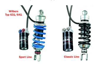
The Wilbers Racing Suspension shock 641 respectively 631 is fitted with a hose connected compression tank. Therefore it is completely and individually tunable in rebound, compression and preload.
