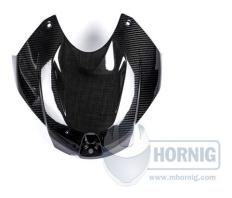
This Upper Tankcover is made of high quality carbon fibre and covered with UV resistant clear lacquer. The article number TAO.204.S100N.K has an ABE/street homologation.
