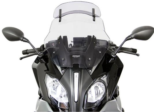
This type of touring windshield has a small spoiler at the top of the wind deflector. Can be manually set to seven positions in terms of angle and height. Tiresome turbulence is also reduced by the air flow at the rear of the spoiler.
