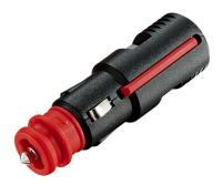
Thanks to its red cap, this plug fits into cigarette lighter sockets (e.g. ZA 01-04). If you remove the red cap, the plug fits into the on-board DIN socket (BMW motorcycle socket).
