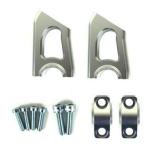
Handlebar risers with offset: 20mm higher and 30mm closer to the rider
