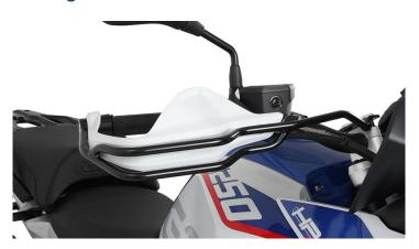
Whether you ride Offroad or on asphalt - this solid hand guard set for the left and the right side reliably protects your hands and your handlebar in case of a downfall. The black powder-coated steel construction is able to withstand enormous pressures, is easy to mount and gives your motorcycle an exciting Offroad look. Only fits vehicles with the original handlebar bracket (if a handle bar riser is mounted, the protection guard may not fit).
