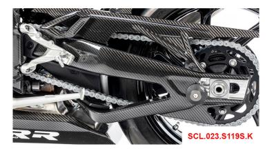
This Swingarm Cover is made of high quality carbon fibre and covered with UV resistant clear lacquer. You have to glue on the carbon fibre covers. We recommend silicon glue.
