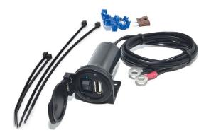
The specially designed USB socket (max. 2,1 A) sets the input voltage from 12V to 5V USB standard. The housing (IPX3) with 1.5 m cable with battery terminals and fuse allows flexible mounting on the handlebars or tubing string with cable ties. A special feature is the comfortable spring cover. The integrated switch On/Off prevents continuous power consumption of the socket, which is indicated by a operation LED.
