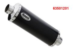
The HURRIC Rac 1 slip-on exhaust impresses with its timeless elegant design as well as with its powerful sound. The elliptical silencer is made of aluminium and is assembled with a screwable mount. The db-killer is removable and the original catalyser will be preserved when mounting the silencer. Colour 63501201: black (anodised aluminum) Height: 125mm Width: 100mm Length casing: 360mm Total length: 445mm
