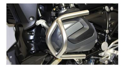
Our stainless steel engine guards will never rust like powder coated steel guards. They are carefully designed to allow clearance for oil changes or valve cover access, so they never need to be removed. Guards attach to the engine mounts not the engine covers to protect the engine heads and not destroy them. Integrated top brackets on each guard allow the rider to mount accessory lights, video cameras, or whatever they can imagine!
