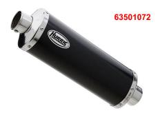
The HURRIC Rac 1 slip-on exhaust impresses with its timeless elegant design as well as with its powerful sound. The elliptical silencer is made of aluminium and is assembled with a screwable mount. The db-killer is removable and the original catalyser will be preserved when mounting the silencer.
