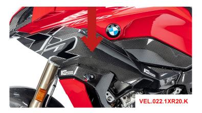
Both side panels are made of high quality carbon fibre and covered with UV resistant clear lacquer. This fairing provides not only a motorsport look but also an advantage in weight!
