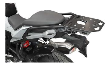
This minirack is a slim, light and inconspicuous luggage solution. Soft luggage can be individually attached to the rear of the motorcycle and lashed thanks to the side slots of this luggage rack. The minirack has a high quality powder coating and a solid construction. A street homologation is not necessary.
