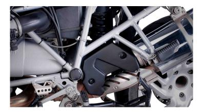
In order to close the lower opening of the frame of your motorcycle and to improve the aesthetic appearance, you have this ABS plastic side panel at your disposal. The aerodynamics of your motorcycle are increased and it is better protected against wind and weather while driving. The side panels are available in black.
