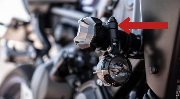
By means of this assembly kit (39mm), the LED auxiliary lights Beam 2.0 can be attached to the crash pad (item 8566N) of your BMW G310R.
