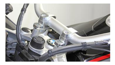
Handlebar risers with offset: 30mm higher and 14mm closer to or away from the rider
