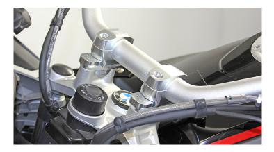
Handlebar risers with offset: 30mm higher and 14mm closer to or away from the rider
