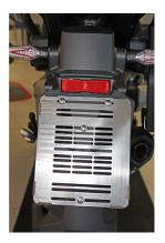
This adjustable licence plate bracket is made of high-quality stainless steel. You can adjust the width from 18 to 28 cm. The height of the licence plate is 20,3 cm.
